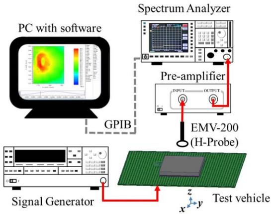
Fig. 4 Measurement setup.
