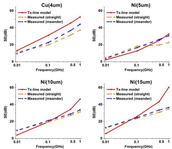
Fig. 5 Measured and modeled SE results with different coating materials.
