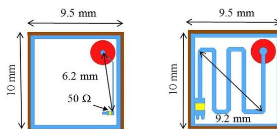
Fig. 1 Configurations of layout patterns: left-handed side is straight-line type and right-handed side is meander-line type.
