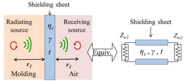
Fig. 3 Schematic of the near-field scenario and its equivalent transmission-line model.
