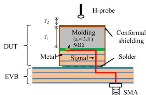
Fig. 2 Structure of the test vehicle.
